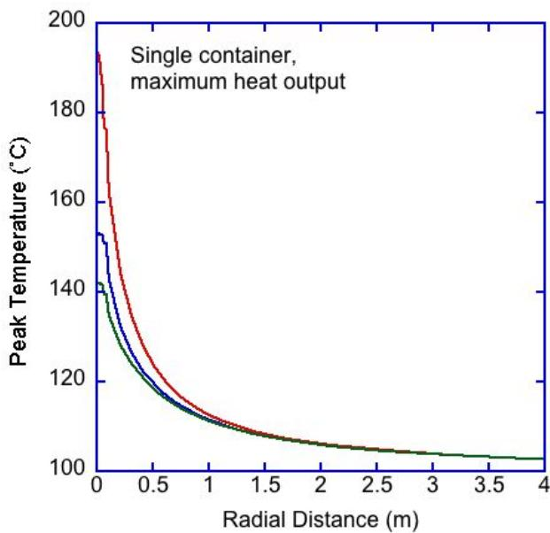
**Fig. 6.2.5** Variation of peak temperature reached along horizontal radii at the top (green), middle (red) and bottom (blue) for a stack of 10 containers, each with two capsules of SrF<sub>2</sub> at maximum heat output
