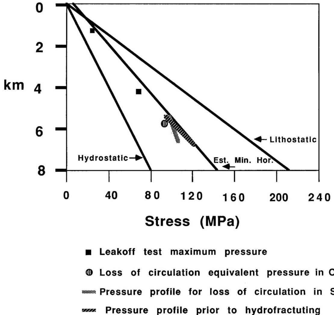
**Fig. 3.3.9** Estimated state of stress in the Gravberg-1 borehole. The points where the formation was actually fractured in sidetrack 3 both during the fluid loss and hydrofracture operation are not known, therefore, a depth range of possible pressures is presented. Stress estimates and figure from /JUH 91/
