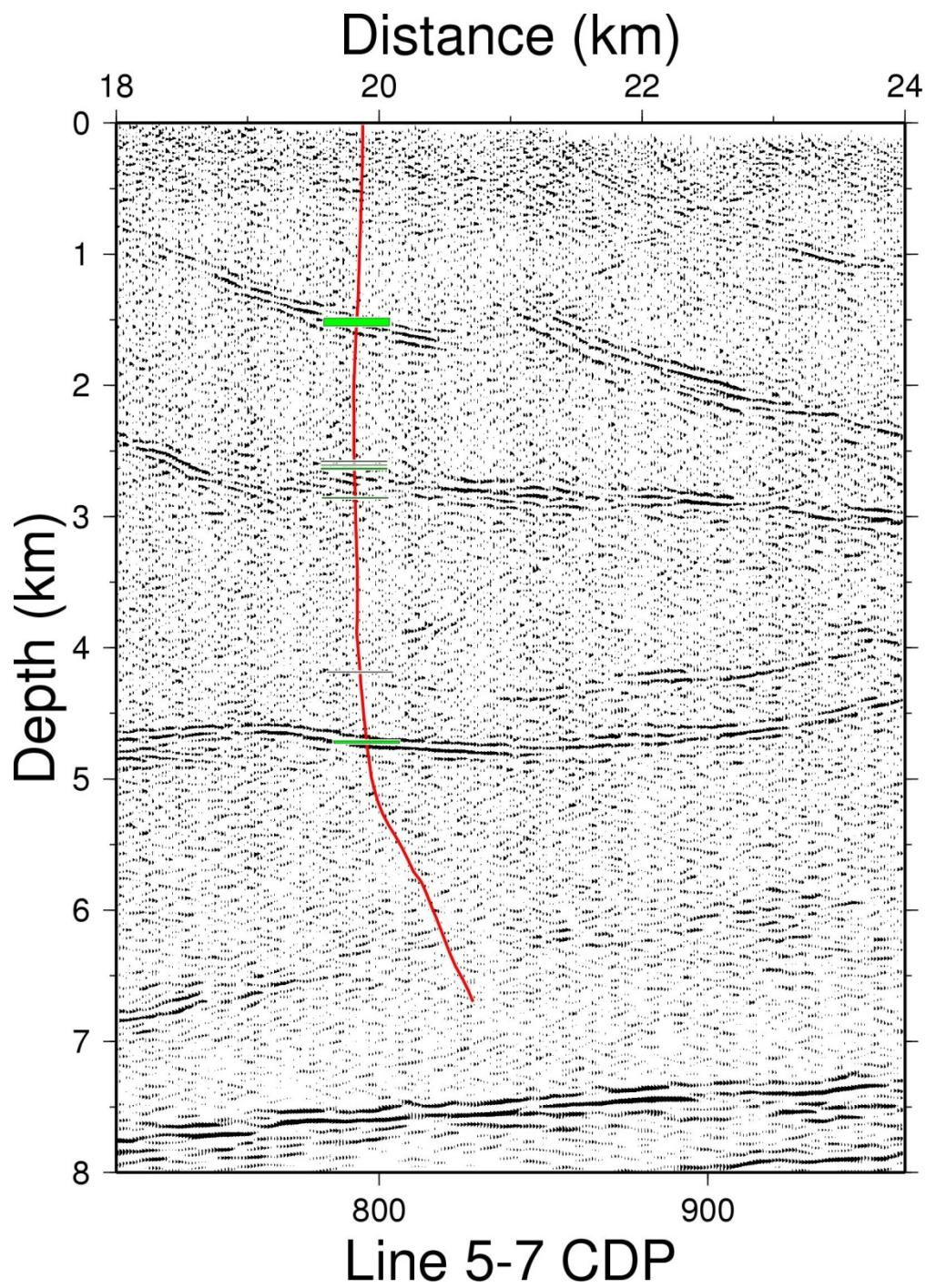
**Fig. 3.3.4** Drilling of the Gravberg-1 borehole shows the marker reflections to originate from thin dolerite sills (green bars) in otherwise granitic bedrock. The data were pre-stack depth migrated. The diffuse reflections intersecting the borehole just below 6 km probably represent thin felsic aplitic intrusions
