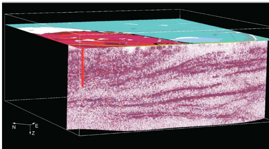
**Fig. 3.3.11** Location of the COSC-1 borehole (red line) on the seismic section. The seismic section corresponds to the site investigation line 2010 in Fig. 3.3.10. The red unit on the geological map is the Seve Nappe and it is highly reflective.
