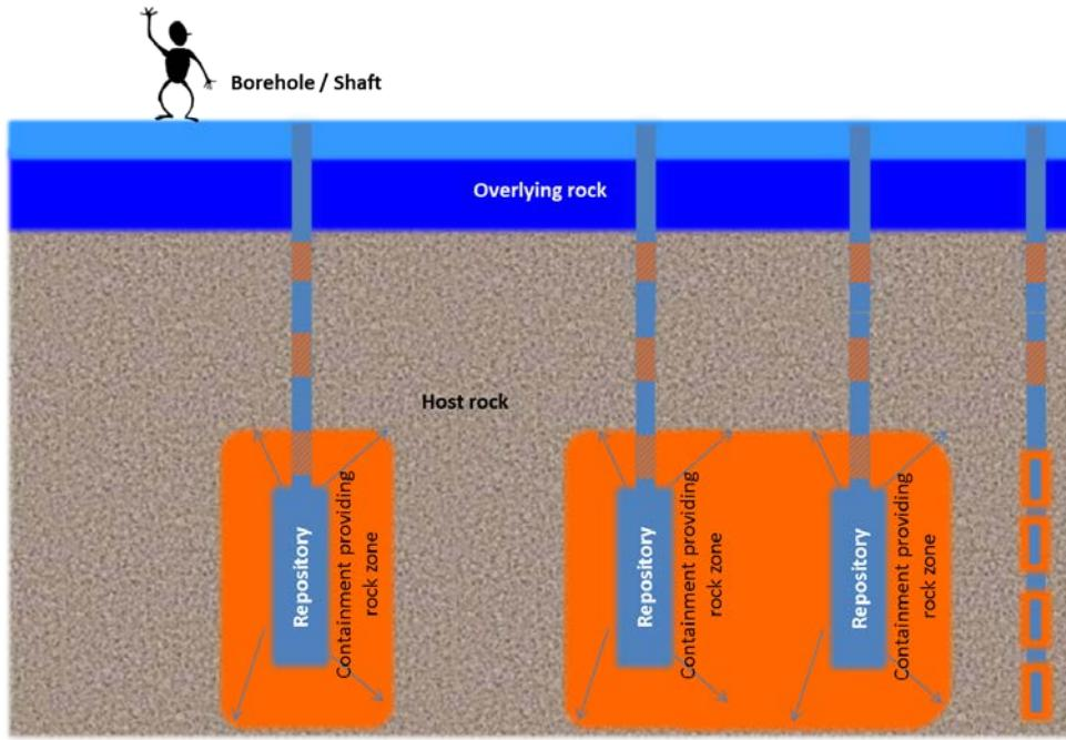
**Fig. 2.3.6** Possibilities for containment providing rock zones for boreholes
