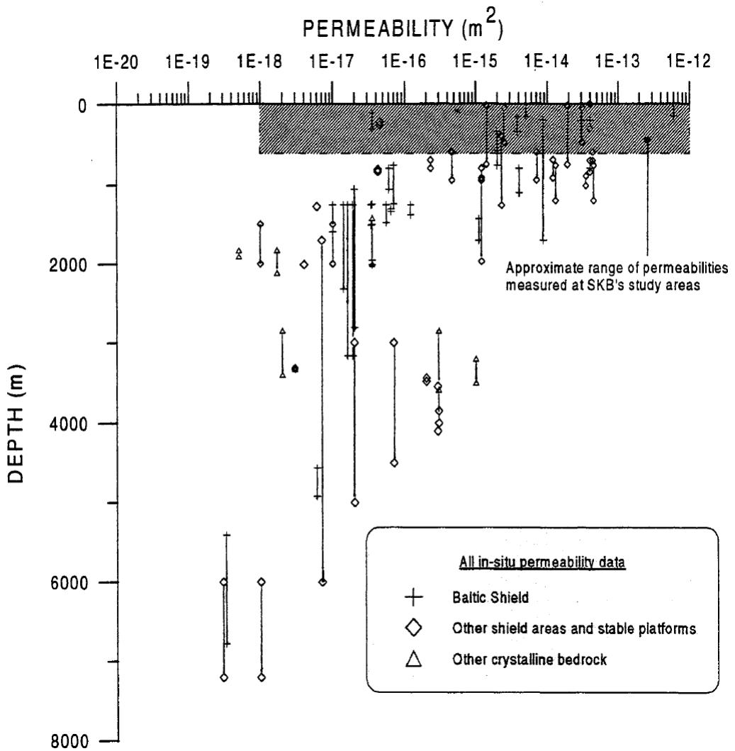
**Fig. 3.3.7** Compilation of permeability measurements in boreholes in the Baltic Shield and other areas. References can be found in /WAL 96/.
