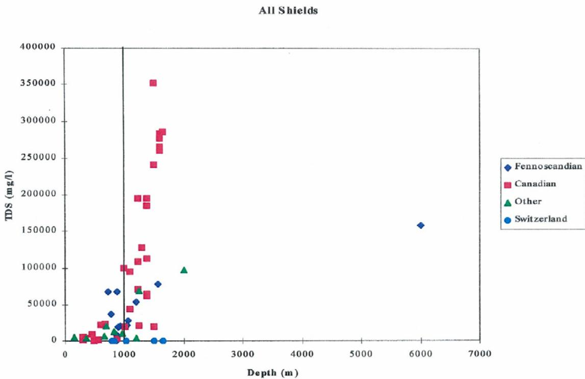
**Fig. 3.3.8** Compilation of total dissolved solids in crystalline rock down to 6 km (from /JUH 98/)
