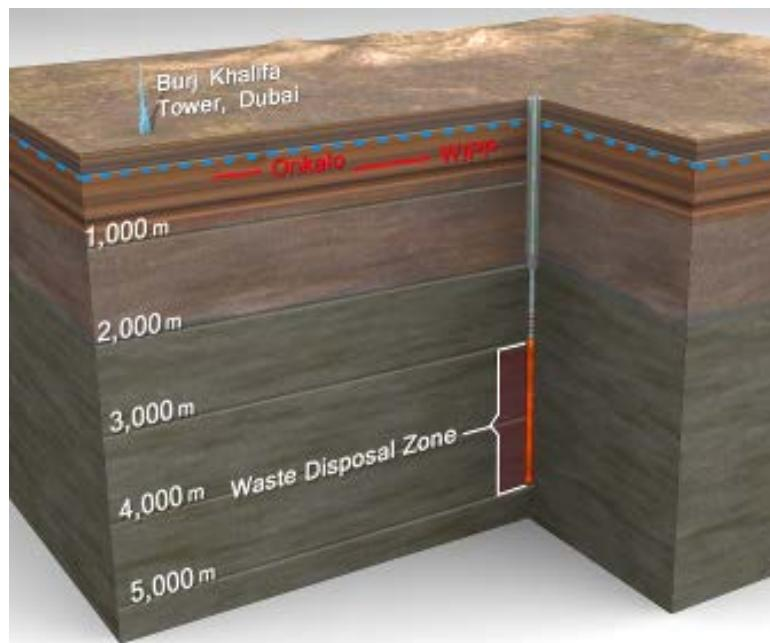
**Fig. 2.2.1** Deep borehole disposal
