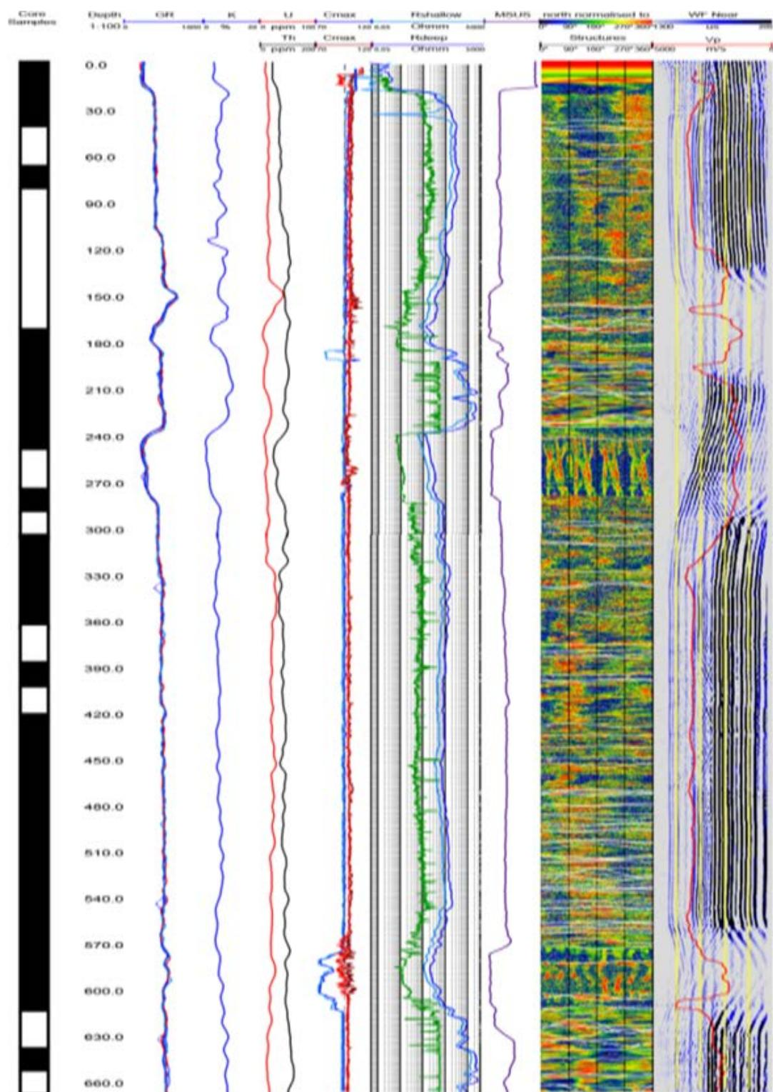
**Fig. 7.1.3** Core recovery (left; black zone core recovery) and summary of downhole log measurements (right, including natural gamma ray, spectrum gamma ray, calipers, resistivity (shallow and deep), magnetic susceptibility, borehole televiewer, and sonic log)
