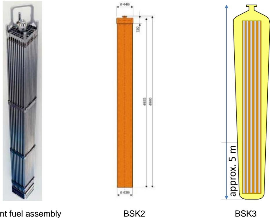
**Fig. 7.2.1** BWR fuel element, canisters BSK2 and BSK3
