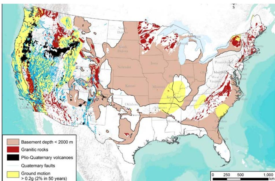
**Fig. 2.2.3** Basement depth, Quaternary faults, volcanic and seismic activity
