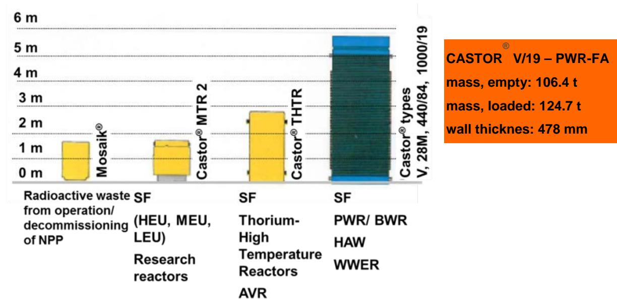
**Fig. 5.2.3** Typical casks for radioactive waste and SF
