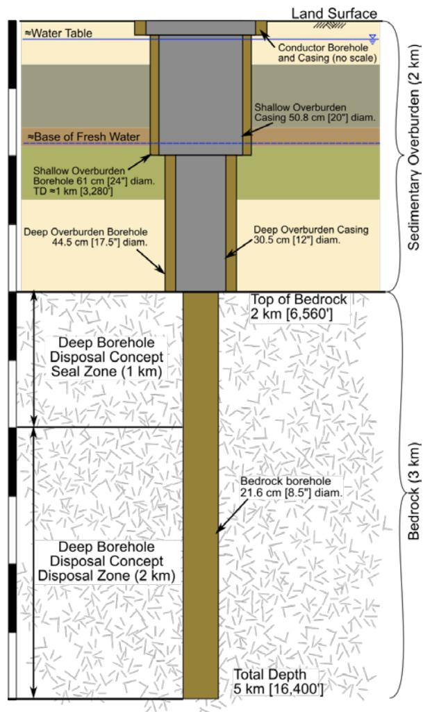
**Fig. 2.2.6** Schematic of characterization borehole.
