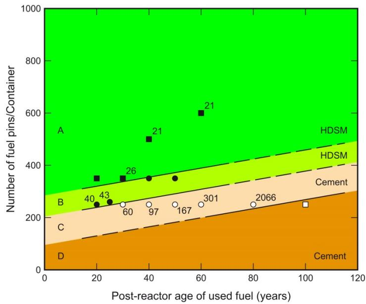
**Fig. 6.2.3** SSM Optimization diagram for a single container of consolidated spent MOX at 65 GWd/t burn-up from the outcomes of heat flow modeling
