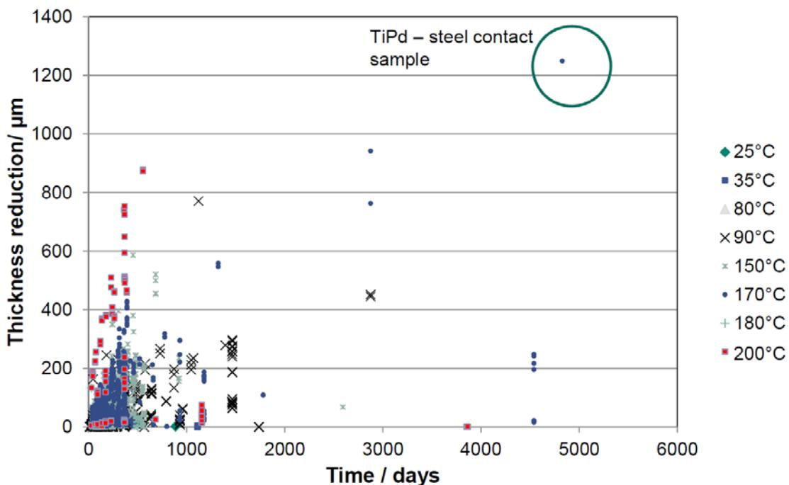
**Fig. 7.2.2** Reduction in thickness of steel plates by corrosion with brines versus time
