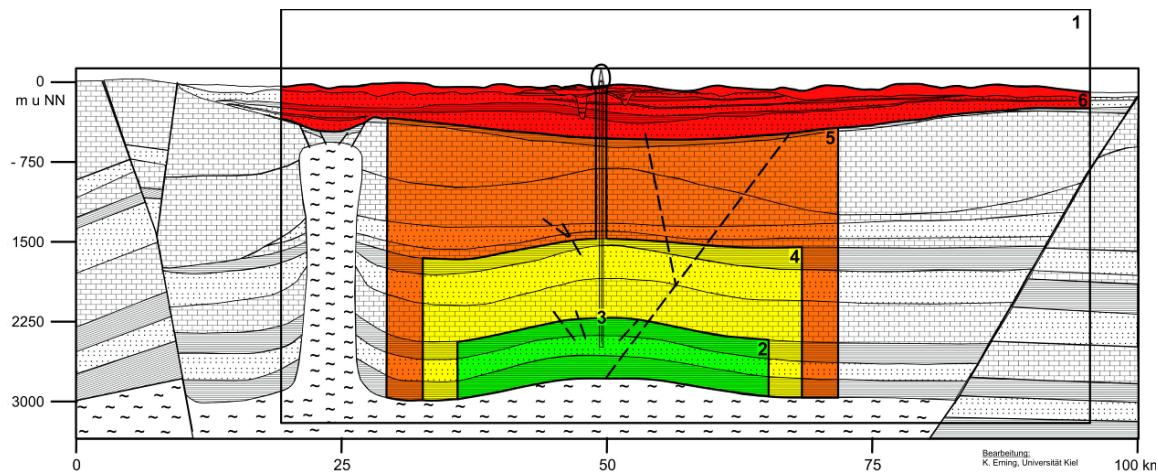
**Fig. 3.4.1** Concept behind multi barrier systems (simplified /GRO 11/). Green: effective containment (storage) zone, yellow: (secondary) retaining formation (cap rocks), orange: transfer-zone consisting of layered permeable and low permeable rocks, red: protected good. Here, an example for a CO<sub>2</sub> storage site is drawn, whereas the CO<sub>2</sub> is deposited within a sandstone.
