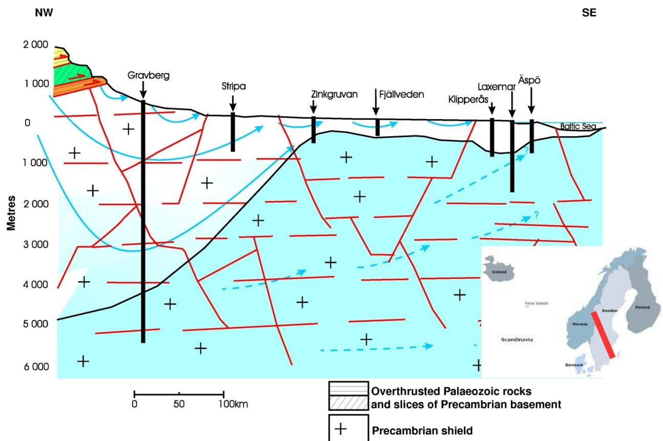
**Fig. 3.3.1** Conceptual model for water circulation patterns along the profile shown by the red line in the overview map. The darker the shading the greater the salinity of the water. Meteoric water is driven deep into the crust by the hydraulic head in the mountains. This model is partly based on earlier work by /LAA 95/.
