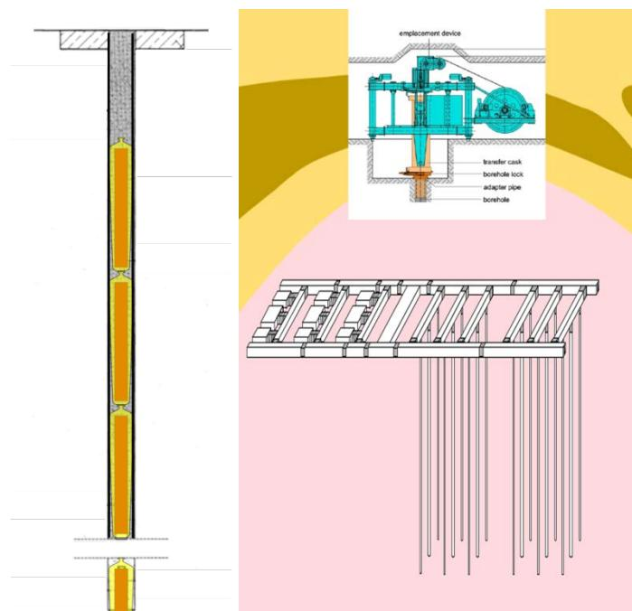
**Fig. 2.3.8** schematical concept of stacking and arrangement of boreholes
