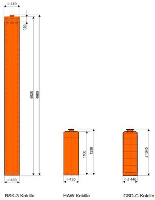
**Fig. 5.2.5** Dimensions of canisters for borehole emplacement
