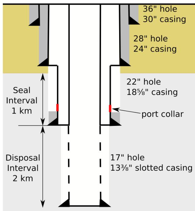
**Fig. 2.2.7** Layout of large diameter borehole
