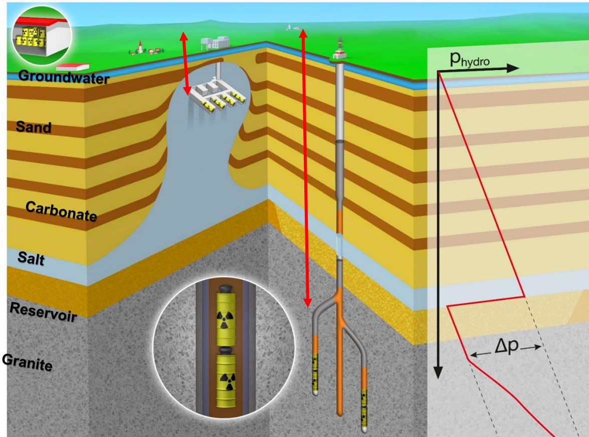
**Fig. 3.4.2** Concept of a multi-barrier deep borehole disposal in comparison to interim storage at the surface (left) and mined repositories (centre)
