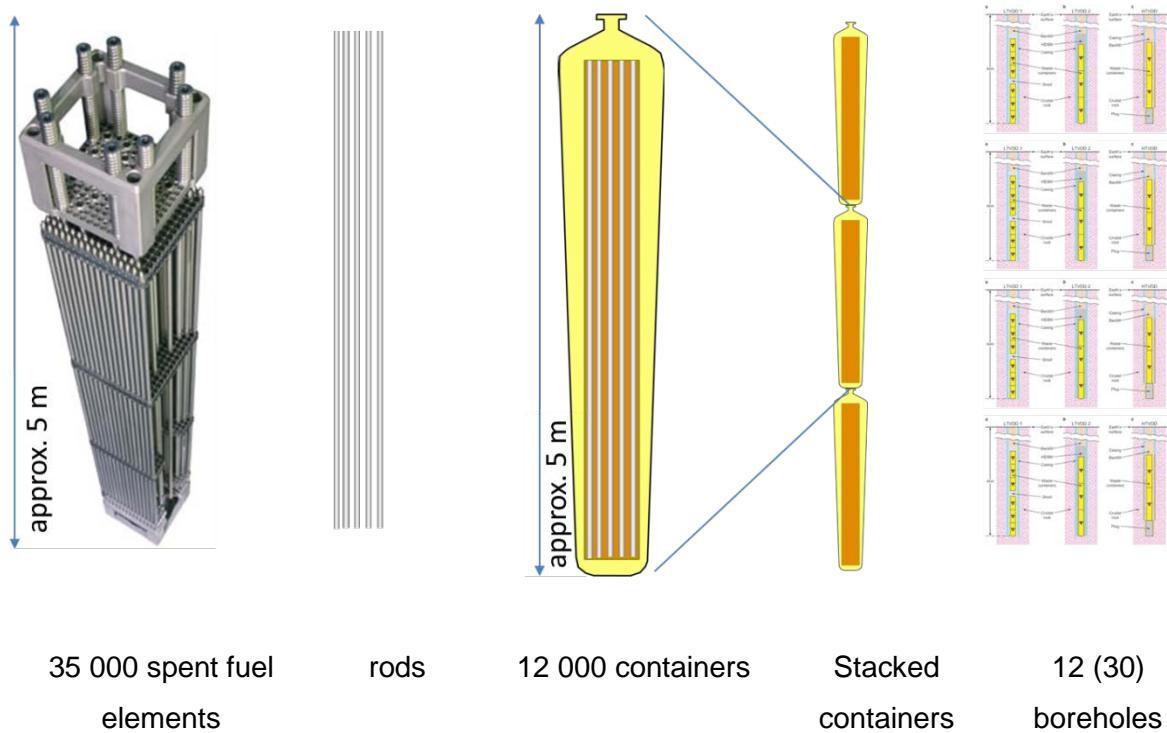
**Fig. 2.3.2** Calculation of number of needed boreholes
