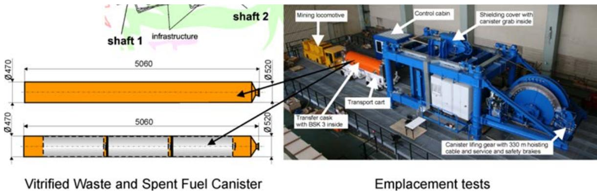
**Fig. 2.3.9** Emplacement device for boreholes
