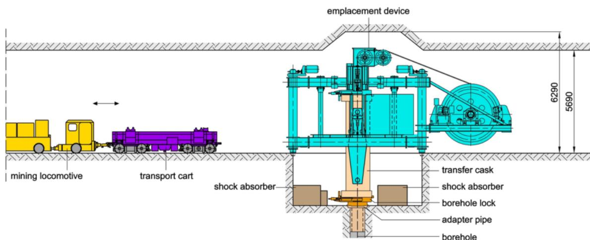
**Fig. 5.2.9** Scheme of the full-scale test equipment for the BSK3 concept
