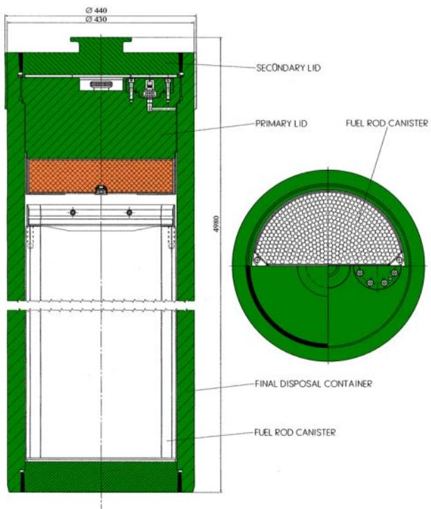
**Fig. 5.2.6** Conceptual scheme of the BSK3 canister
