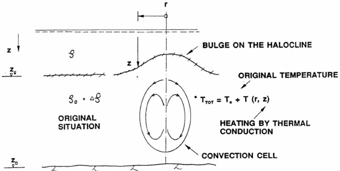
**Fig. 3.3.2** Bulge on the halocline due to temperature increases from the stored spent fuel. If the density contrast is large enough between the water above and below the halocline then no saline water will circulate to the surface. (From /LAA 95/)
