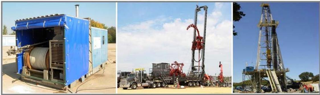
**Fig. 6.1.1** Wireline unit for logging or fishing on cable (left, a coil-tubing unit for well work-over and fishing with CT pipe (center) and a 1 million pound hook load capacity „heavy“ oilfield drill rig for drilling deep boreholes and fishing with pipe (right)
