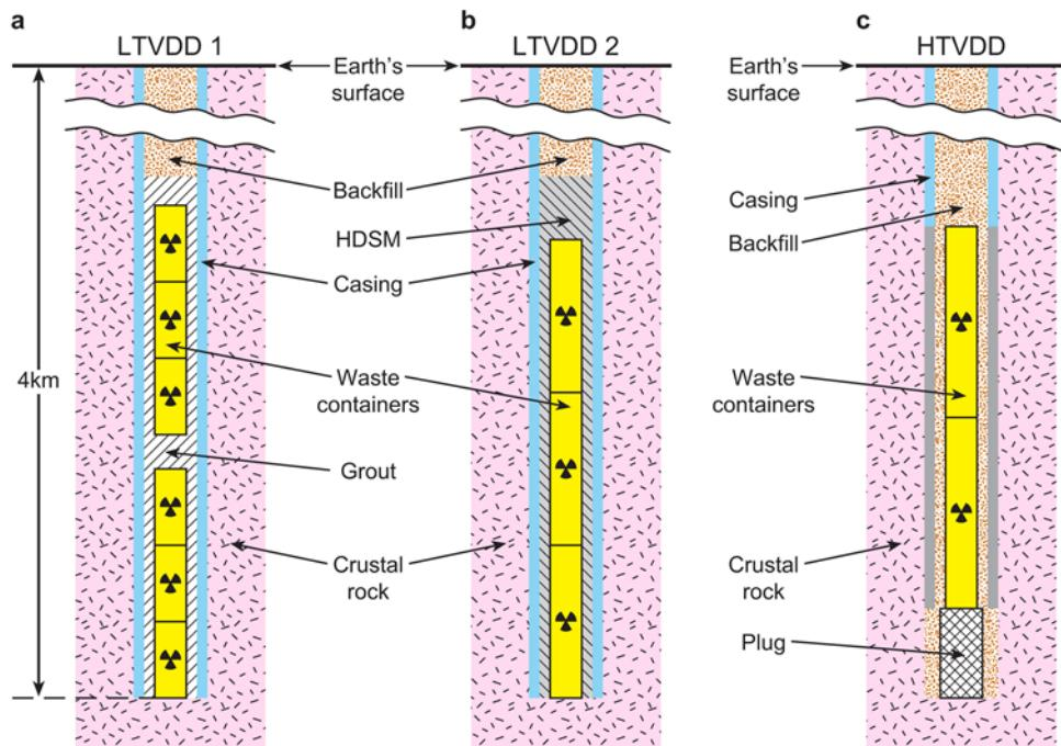
**Fig. 6.2.1** Three design concepts for DBD: HDTVDD, LTVDD1 and LTVDD2. (Note – the outer annulus between the casing and host rock is not shown.)
