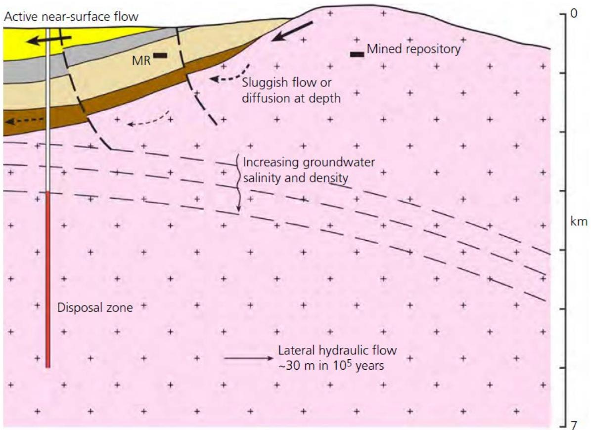
**Fig. 7.2.3** Schematic sketch for disposal in a borehole and a mined repository in a granitic environment (graph taken from /BES 14/)
