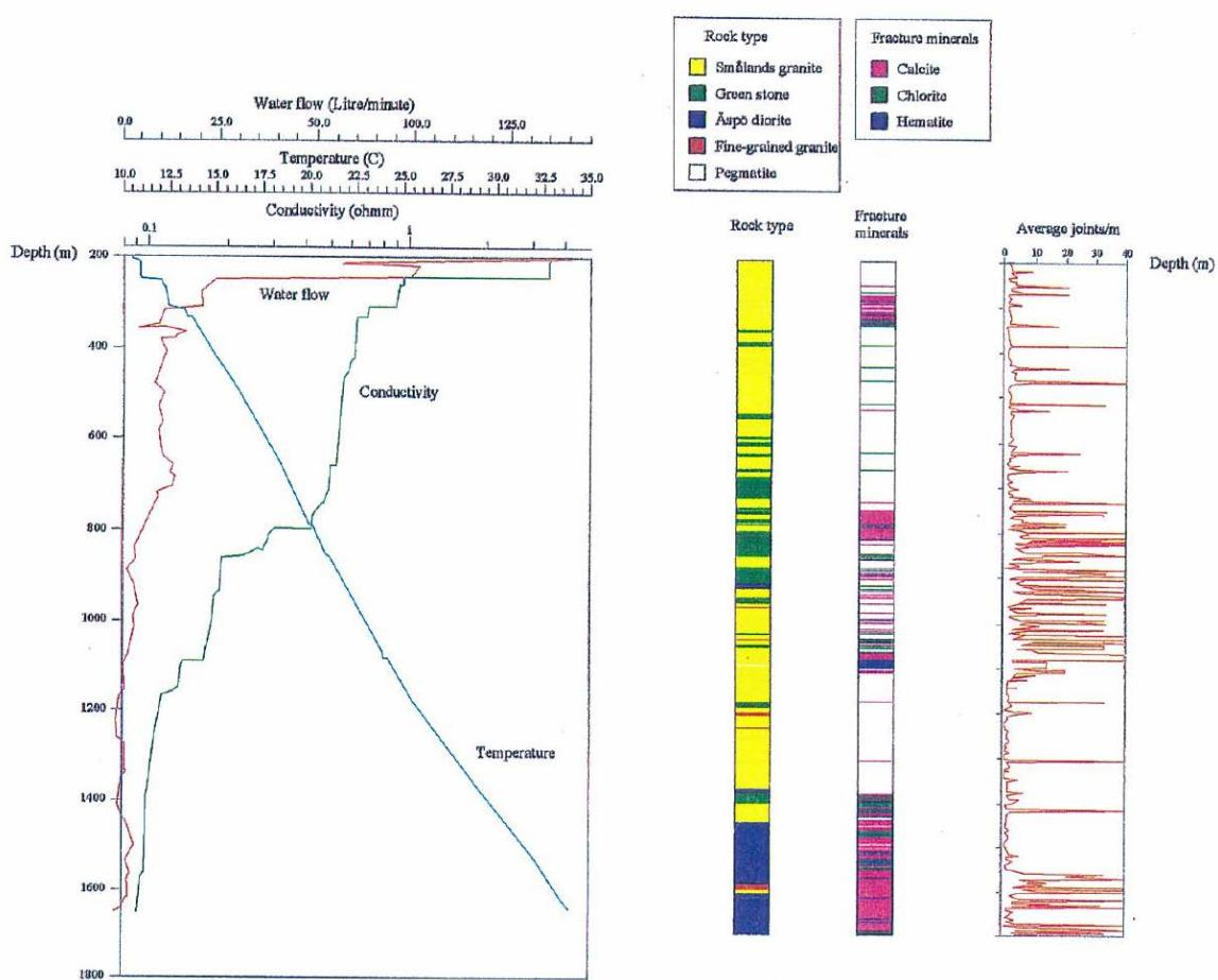
**Fig. 3.3.5** KLX02 downhole groundwater logging profiles and lithological, fracture frequency and fracture mineral data (from /LAA 95/). Note the intense fracturing at 700 to 1100 m and below 1560 m. Laxemar is located at the southern end of the red line in Fig. 3.3.1. (From /JUH 98/)
