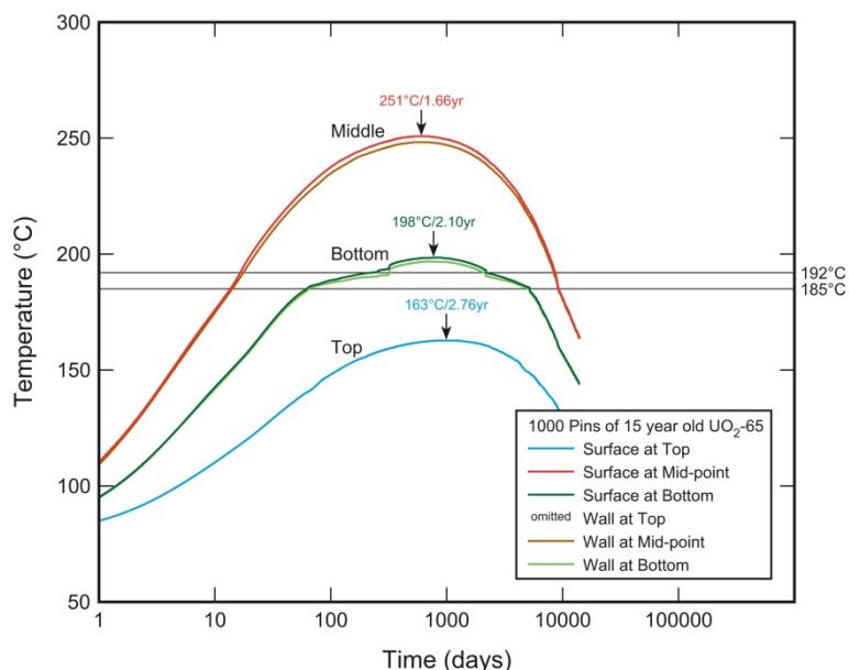
**Fig. 6.2.2** Variation of temperature with time at the outer edge of the waste package and at the borehole wall for three levels (top, middle and bottom) for a single container of consolidated spent UO<sub>2</sub> (65 GWD/t burn-up). Horizontal lines show the solidus for the HDSM at 1 atmosphere and 50 MPa (projected)
