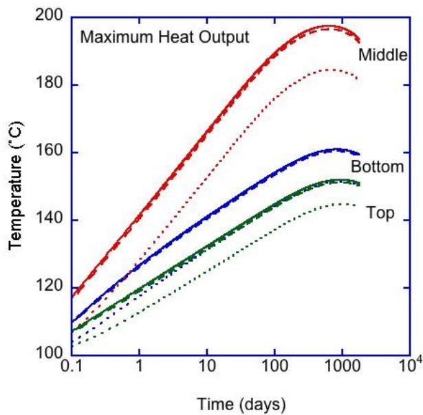
**Fig. 6.2.4** Temperature time curves for disposal of a stack of 10 containers of  $\text{SrF}_2$  at maximum heat output
