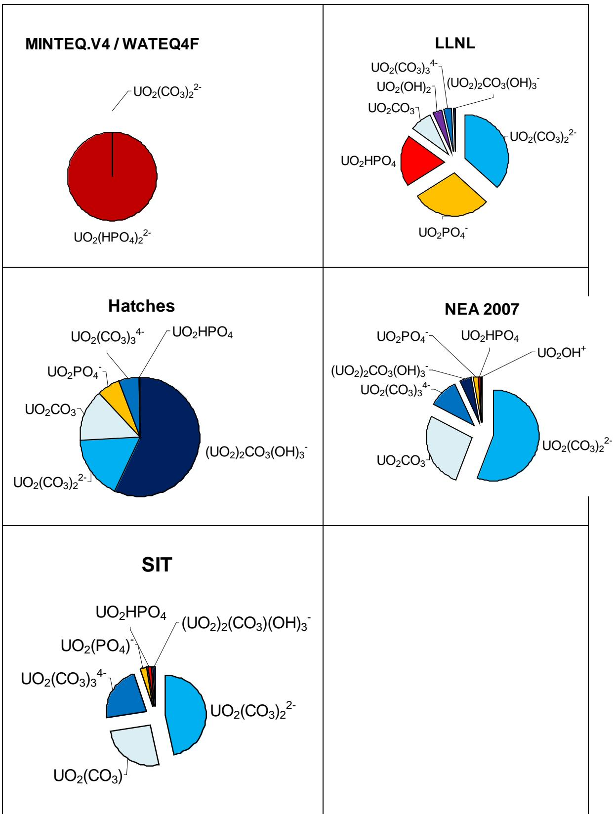
**Fig. 7.4.2** Speciation of uranium based on the data from Figure 1 (12 °C, pH 6.5, pressure 0.1 MPa and different databases using PHREEQC 3.06
