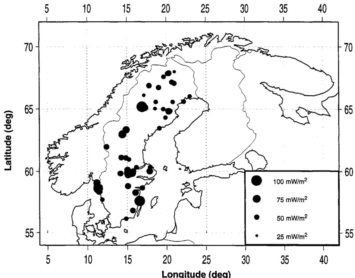
**Fig. 3.3.6** Location of heat flow measurements in Sweden and corresponding values.
