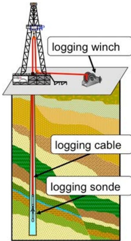
**Fig. 7.1.1** Downhole logging scheme
