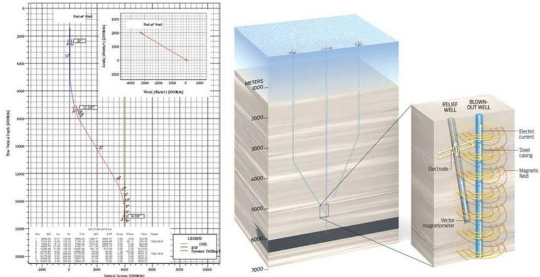
**Fig. 6.1.3** Directional drilling planning of a relief well in the vertical projection (left) and 3-dimensional position towards the target well (center) with the final approach section with home-in wire-line logging (right)
