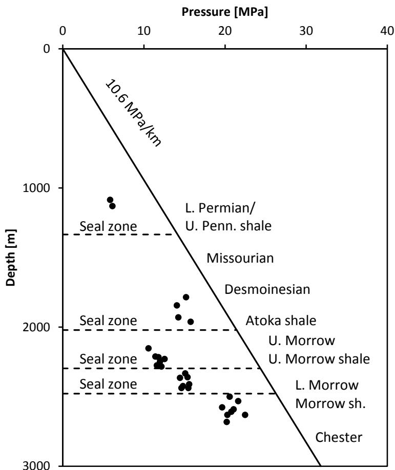
**Fig. 3.4.4** Natural pressures are sealed against each other for millions of years vertically. The example shows a pressure-depth profile from Beaver County (Oklahoma) that illustrates numerous differently underpressured compartments. Redrawn after /PUC 03/
