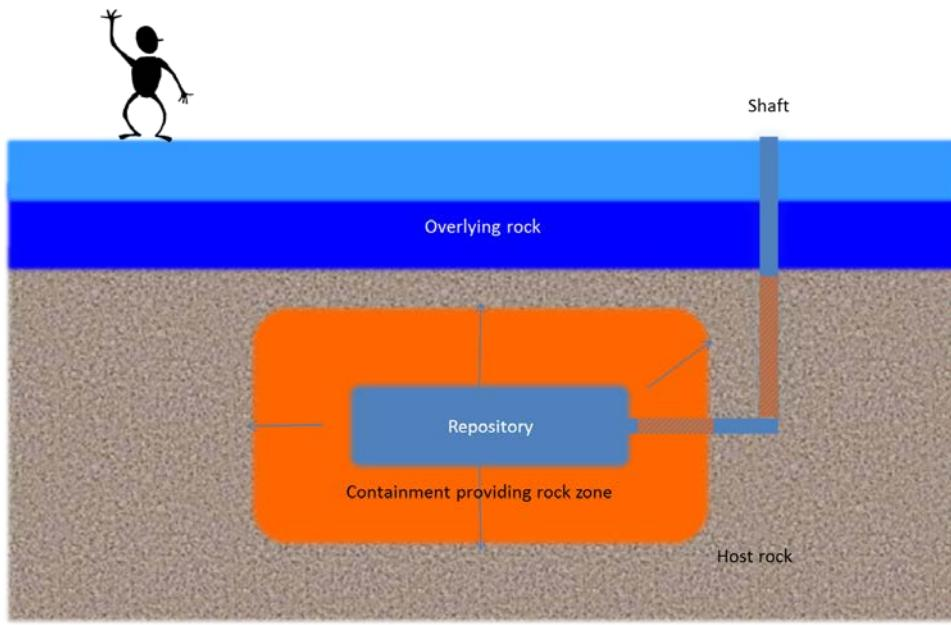
**Fig. 2.3.5** Containment providing rock zone for a geological mine
