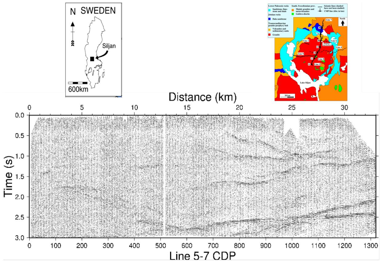
**Fig. 3.3.3** Location of the Siljan Ring area in Sweden, simplified geological map and composite seismic section of the north-south striking lines 5 and 7. The Gravberg-1 borehole is located at a distance of about 20 km (CDP 800). See Fig. 3.3.4 for a depth section in the vicinity of the borehole.
