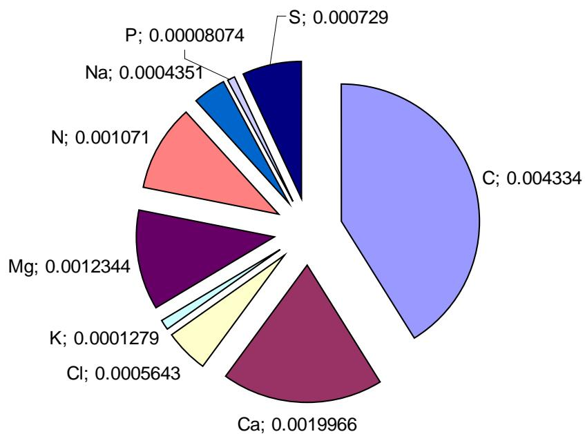
**Fig. 7.4.1** Assumed chemical composition of a groundwater (mol/L) with respect to major cations and anions plus uranium (200 µg/l) and arsenic (25 µg/L) not shown in the diagram
